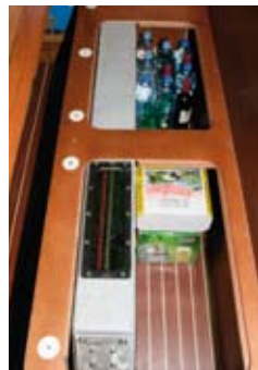
BELOW: Centreboard control lines are visible and replaceable through the water-level Perspex panel
